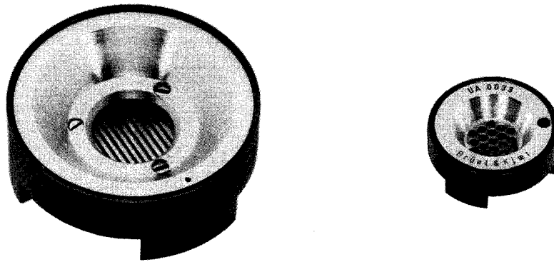
Fig.7.1. Electrostatic Actuators UA 0023 (one-inch) and UA 0033 (half-inch)
